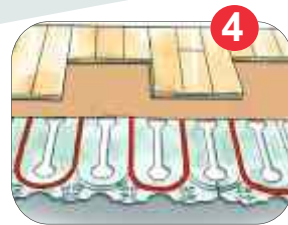
4 Lay underlayment padding and then floor covering
